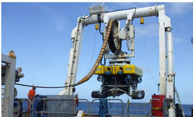
Figure 9 – Umbilical trencher on board MV Emerald Sea.
