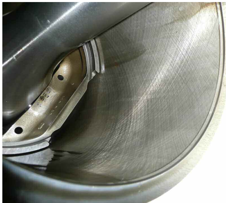
The cylinder inspection showed that all honing marks were clearly visible. No bore polishing or lacquering was noted.
