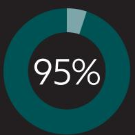
Base oil comprises up to 95 percent (by weight) of grease. Base oil may be mineral oil, synthetic oil or any fluid that provides lubricating properties; however, all aviation greases use synthetic base oil. It is the base oil component that performs the actual lubrication, except in very slow or oscillating applications.
