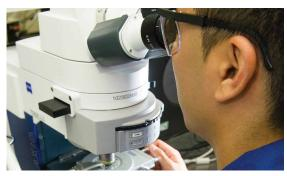
Low-temperature optical microscopy aids in understanding wax crystallization behavior.
