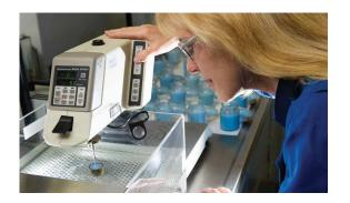
A lab technologist positions a needle until it just scrapes the surface of the wax in preparation for the ASTM D1321 penetrometer test, which measures the hardness of a wax.
