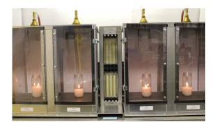
Our custom-designed burn chamber provides a controlled environment to evaluate a candle's burning characteristics.
