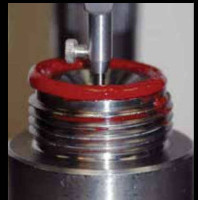
75/25 grease mixture (Mobil Aviation Grease SHC 100 and Unirex S2) Penetration after rolling
