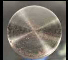
Commercial AD Monograde claiming to meet the Lycoming antiwear-antiscuff additive requirement (SAE 50)
