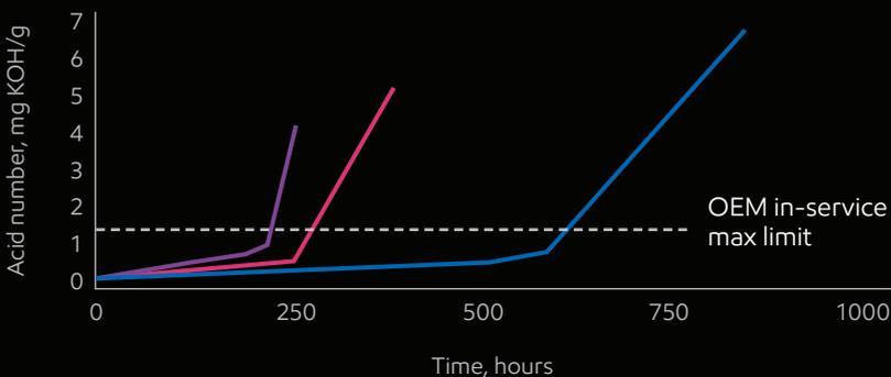
**Hydraulic fluid life (Ampoule test @ 0.5% water, 125°C)**
