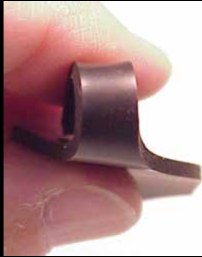
The fluorocarbon elastomer specimen exposed to Mobil Jet Oil 387 lubricant is pliable and shows no cracks.
