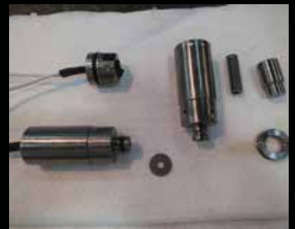
IDG oil pressure switches malfunction when diodes fail due to inadequate oil conductivity.
