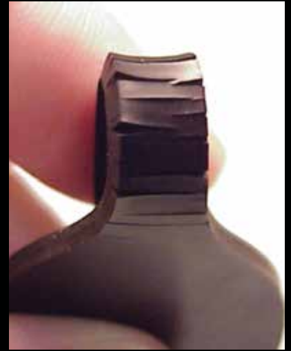
The fluorocarbon elastomer specimen exposed to competitive HPC oil is brittle with visible cracks.
