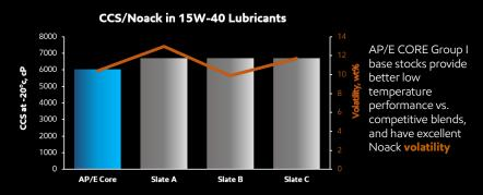
Based on Market General approved API CI-4 additive package. SAE15W-40 lubricants blended at equivalent KV100°C and CCS-20°C
