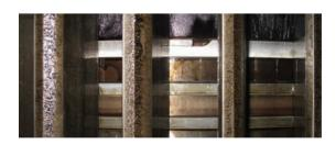
After 8,000 hours, the Jia Run's pistons, piston rings and liners were free of deposits and exhibited negligible wear.
