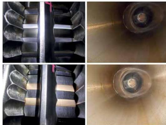
The liner wave cut marks were still clearly visible on all units
