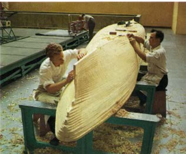
Hand-forming a hull model made of wood in the Model Manufacturing shop. Models are also made from paraffin wax and in special cases glass-fibre laminate. This shop has a hull profiling machine for wax and wood.
