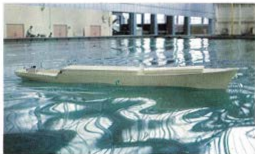
Close-up of a free-running model being studied for its sea-keeping ability.
