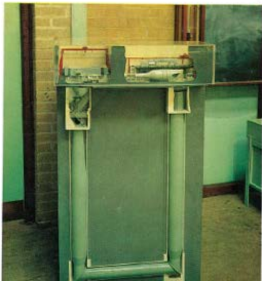
Model of the Water Tunnel used for propeller and hydrofoil design research. Impeller section is left. Water is taken down 180 ft. below measuring center and subjected to high pressure to keep air content of the water constant.
