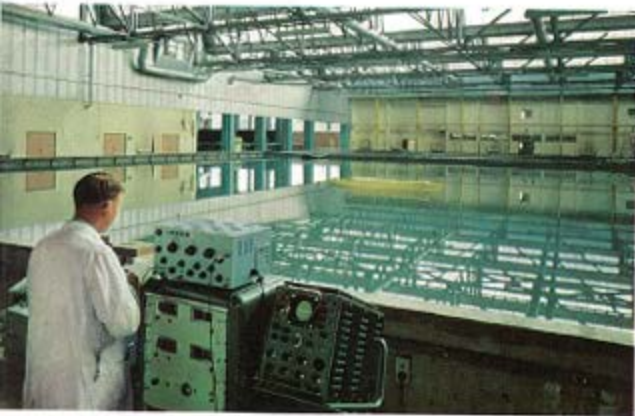
Maneuvering Tank with model ready for test. Gear foreground remotely controls free-running hull under study. Data from test is either recorded on model or telemetered ashore. Aft of the opposite shore is the Model Storage Tank.
