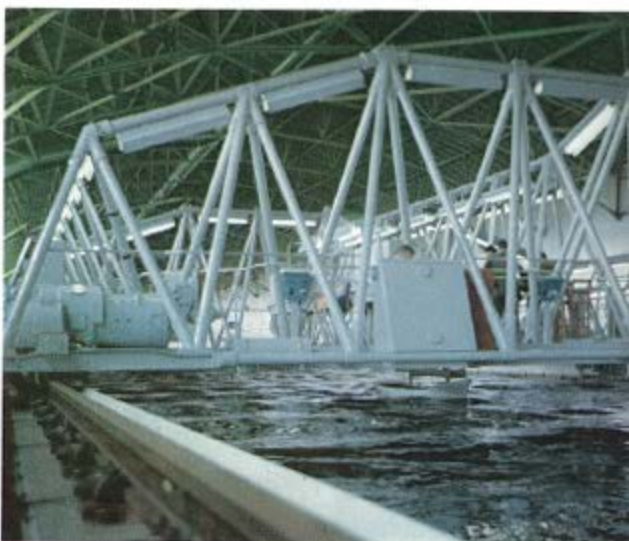
Main tank and towing carriage with hull model under test. Note beach system in tank's opposite shore. Scientists aboard carriage are reading instrumentation to check hull's performance.
