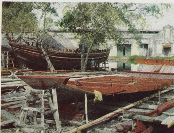
Junks are built without blueprints using techniques handed down from father to son and only minimum "chips" tools. Note hand hewn ribs (lower right). Background is Singapore's Alexandra Canal.
