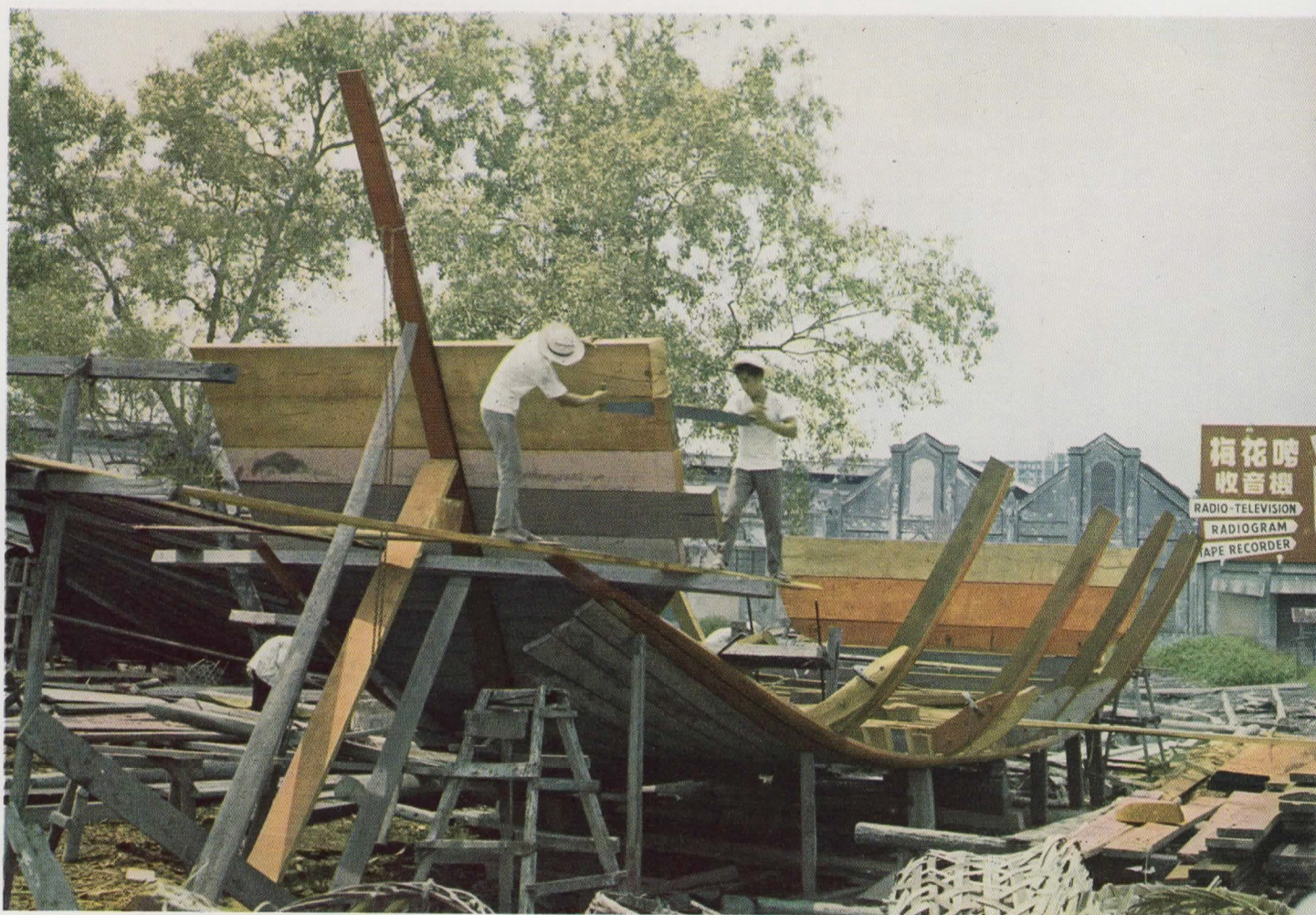
Hand fashioning stern to fit planking contour. Note rib installation.
