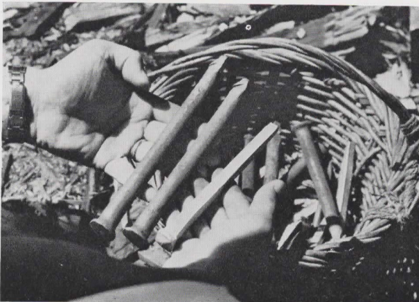
Iron pegs with barbed ends or aluminum pegs are used to fasten strakes to ribs.
