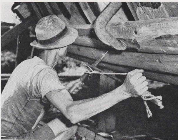
Ancient Chinese fiddle drill in operation.
