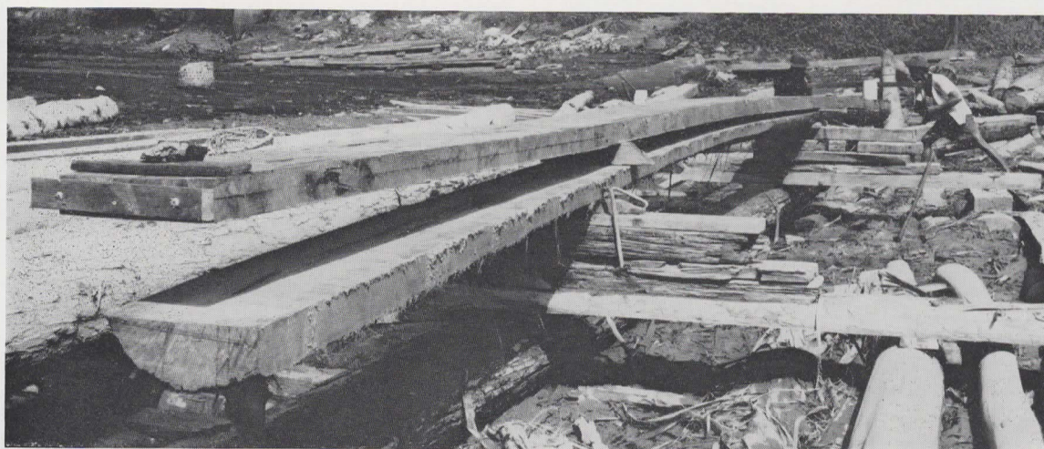
Kayu gam logs are hand sawn along grain using push-pull type saw. Water is used to lubricate saw drips continuously from the white can atop log.
