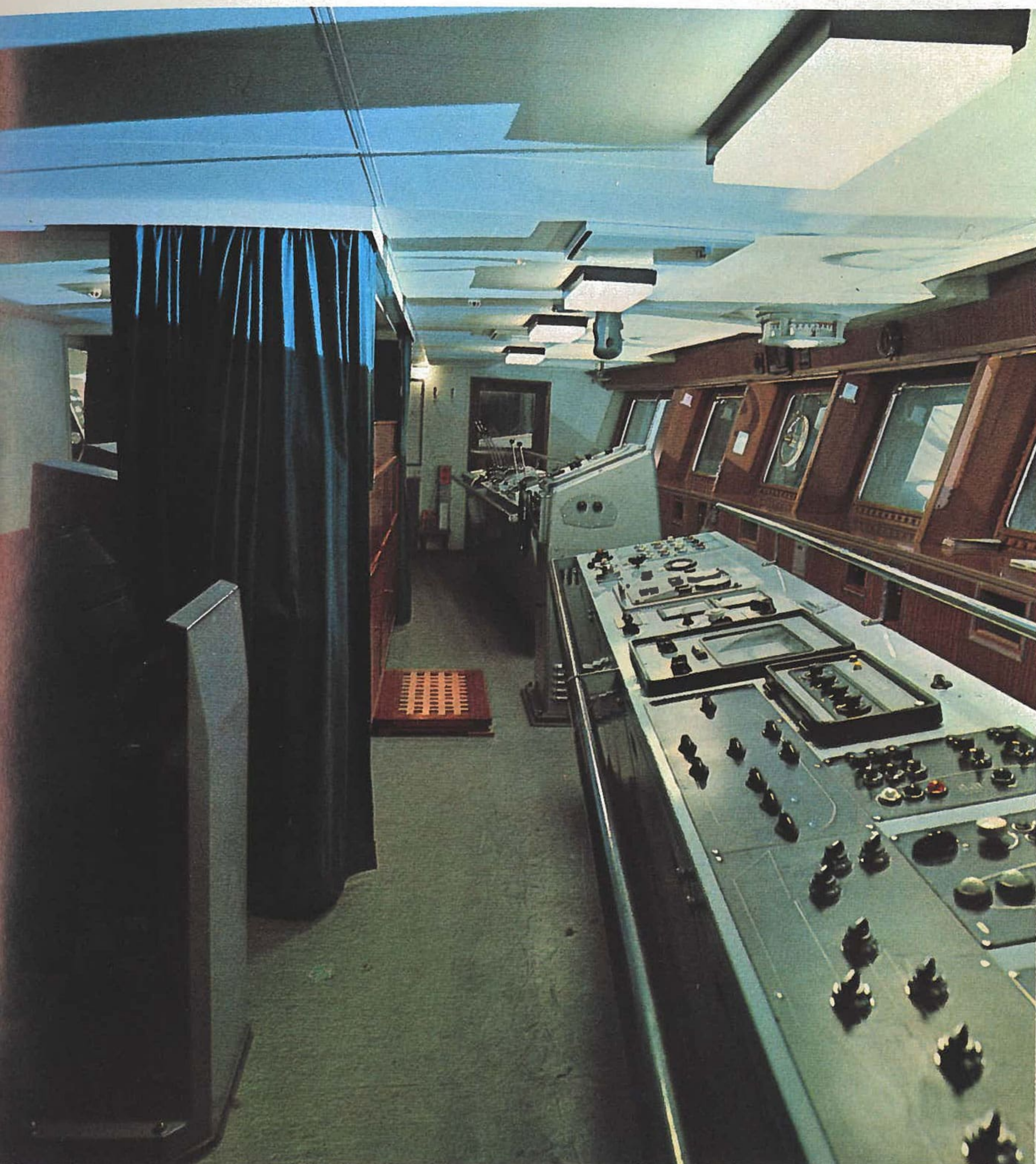
Left—Bridge has all latest navigating gear including remote controls for the main engines
