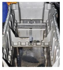
**Engine oil pan:**Very little to no sludge buildup
