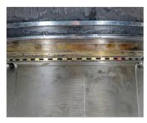
**Pistons:**No evidence of stuck rings or clogging of the oil ring; all rings had normal face wear
