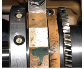
Oil gear pump: Minimal to no wear present
