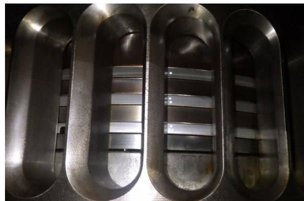
Fig 1 Pre IMO 2020 Using HSFO and Mobilgard 5100 Unit 3 exhibits high level of cleanliness without observable deposit (Dec 2019)
