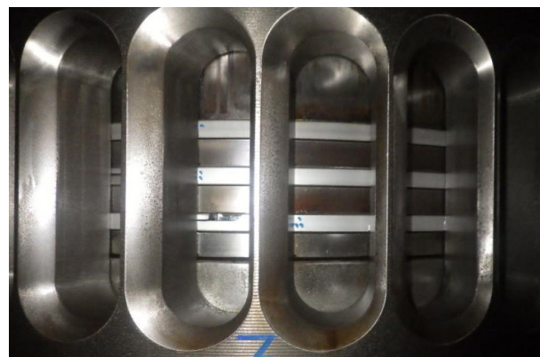
Fig 2 Post IMO 2020 Using VLSFO and Mobilgard 540 Unit 3 continues to exhibit high level of cleanliness after 2500 hr use of Mobilgard 540 (Jun 2020)
