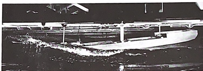
Striking high-speed photograph showing how model test hull reacts to man-induced seaway.
