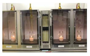
A custom-designed burn chamber provides a controlled environment to evaluate a candle's burning characteristics.
