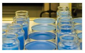
A standardized internal appearance test has been used extensively to assess quality attributes such as adhesion, frosting, and top shrinkage.
