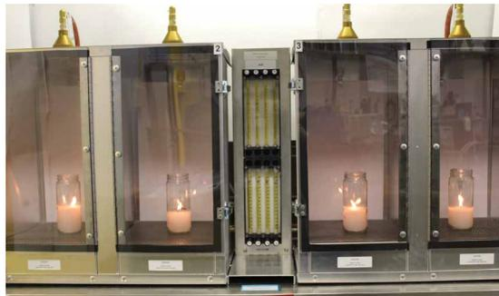
A custom-designed burn chamber provides a controlled environment to evaluate a candle's burning characteristics.
