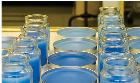
A standardized internal appearance test has been used extensively to assess quality attributes such as adhesion, frosting, and top shrinkage.
