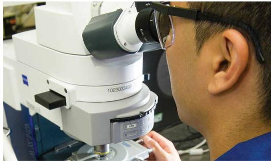
Low-temperature optical microscopy aids in understanding smooth wax crystallization behavior.
