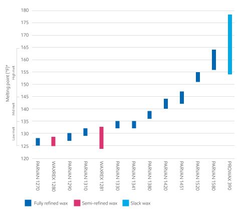
\* Melting point by ASTM D87 except for Prowax 390 with ASTM D938
